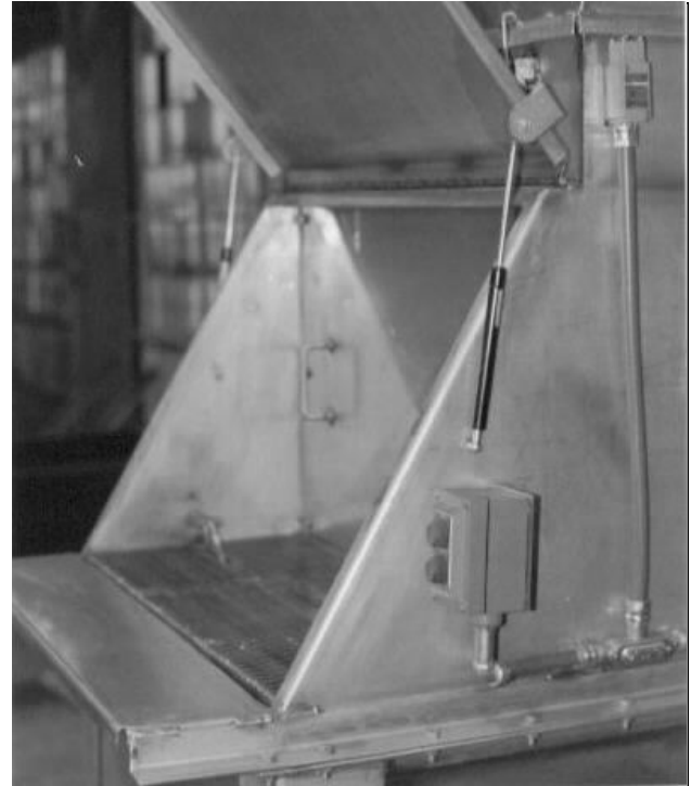
Stainless steel bag dump station with push button operator's controls and support legs to grade
