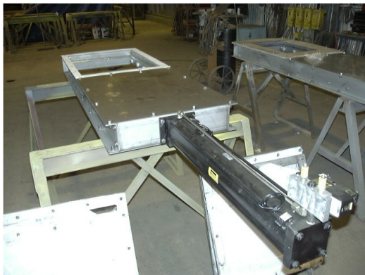
Large horizontal gate valves for granulated sugar service. Throat opening is ~ 36" square. All contact surfaces are T-304L-SS construction, with heavy-duty double-acting air cylinder actuation.
